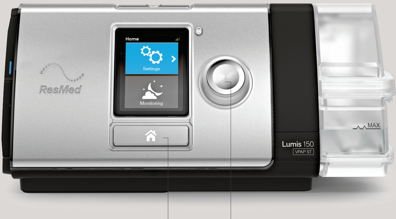
Hold down the home button and dial together for three second to unlock the Clinical Menu
